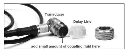
When measuring, press against the top of the transducer with the thumb or index finger to hold the transducer in place. Moderate pressure is sufficient, as it is only necessary to keep the transducer stationary, and the delay line seated flat against the surface of the material being measured.
